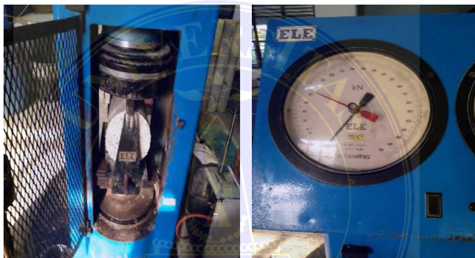
Gambar 3.3. Alat Uji Tekan Beton ( Universal Testing Machine ) Sumber: Penelitian Laboratorium, 2018
