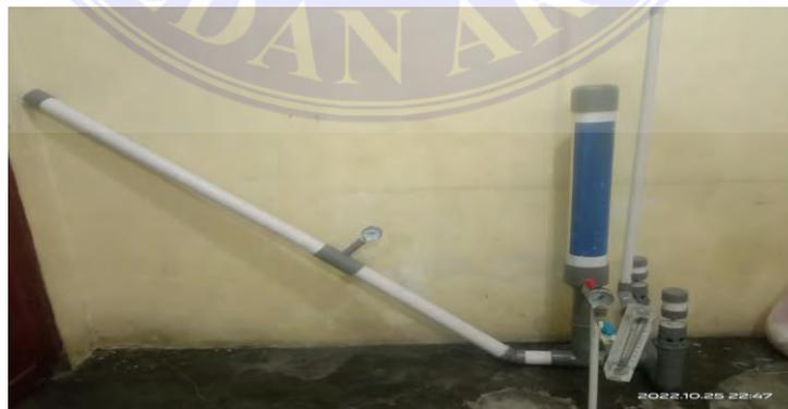
Gambar 3.1. Pompa Hidram Double Katup
