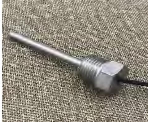
Gambar 3.9. *Stainless Steel Thermowell*
