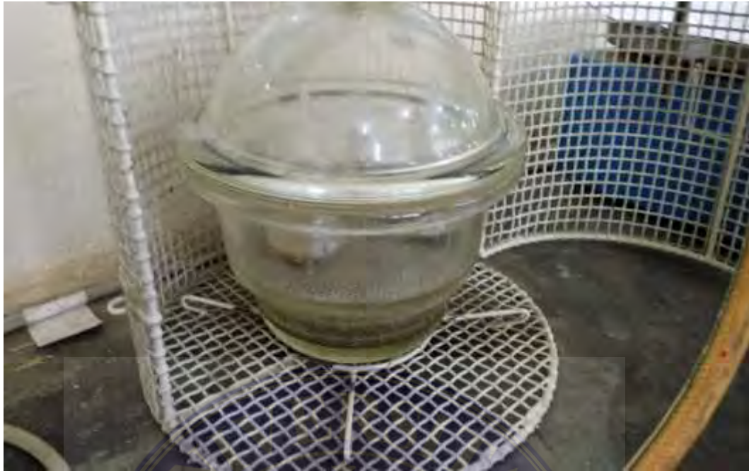
Gambar 5.7 Tahap Vacuum specific Gravity Gs Sumber : Data laboratorium POLMED ,2018
