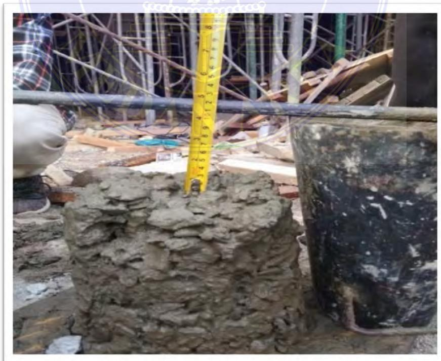
Gambar 16: Uji Slump Test
