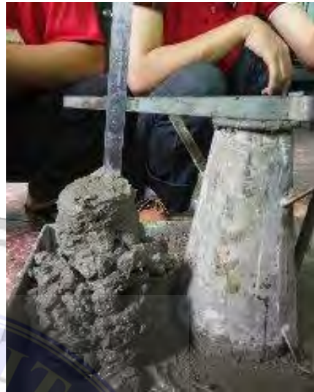
Uji Slump Beton
