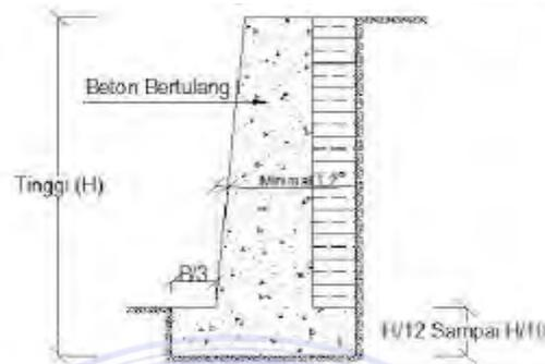
**Gambar 2.2** Dinding Penahan Tanah Type Kantilever (*Cantilever retaining wall*)
