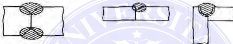
(b) Partial Penetration Groove Welds
