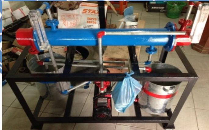
Gambar 3.1 Alat penukar kalor shell and tube
