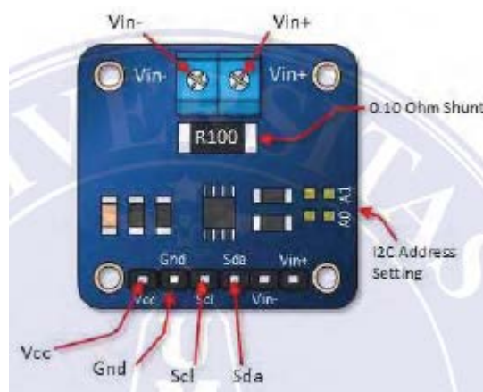
Figure 2.4. INA219 Sensor
