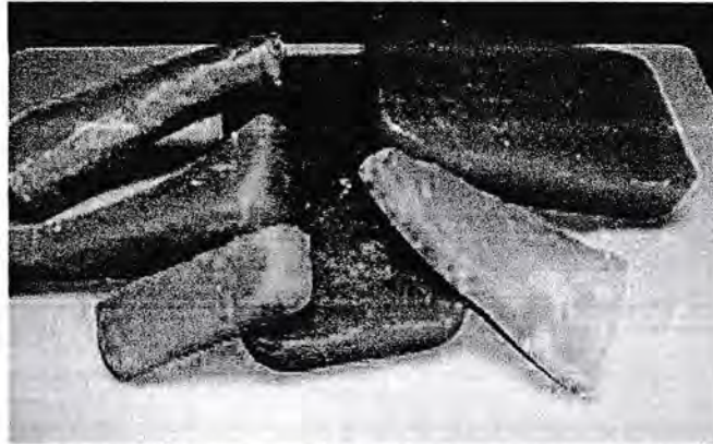
Fig. 2 Paraffin wax as thermal energy storage material
