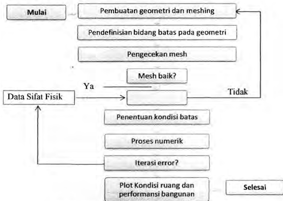
Gambar 3.2 Diagram alir proses simulasi CFD
