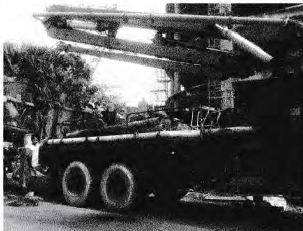
Gambar 20. Concret pump
