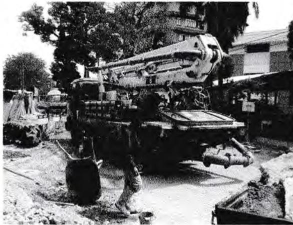
Gambar 19. Concret pump
