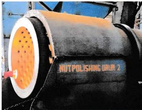
Gambar 3.10. *Nut Polishing Drum*
