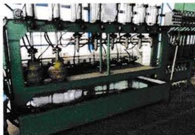
**Gambar 3.35 Visual Mesin *Hydrostatic Test***
