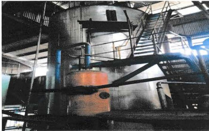
**Gambar 3.13** *Continuous Settling Tank (CST)*
