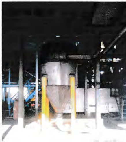
Gambar 3.17 Sand Trap Tank
