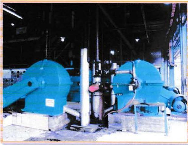
**Gambar 3.35** Sludge Centrifuge
