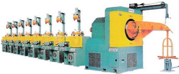
**Gambar 3.7. *Wire Drawing Machine***
