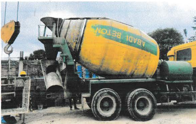
Gambar 3.2.8 Beton Ready Mix
