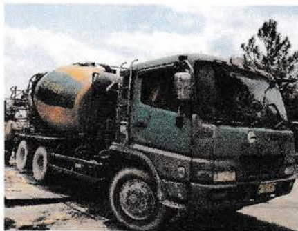
Gambar 3.9 Truck Concrete Mixer Sumber : data lapangan
