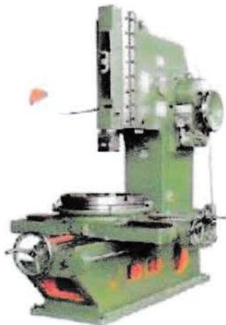
Gambar 3.11 Mesin Bubut *Vertical Turning & Boring Milling*
