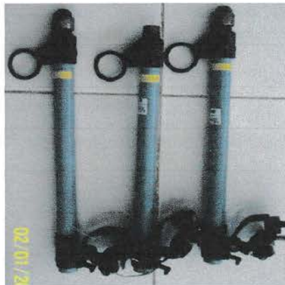
Gambar 3.2 Fuse Cut Out
