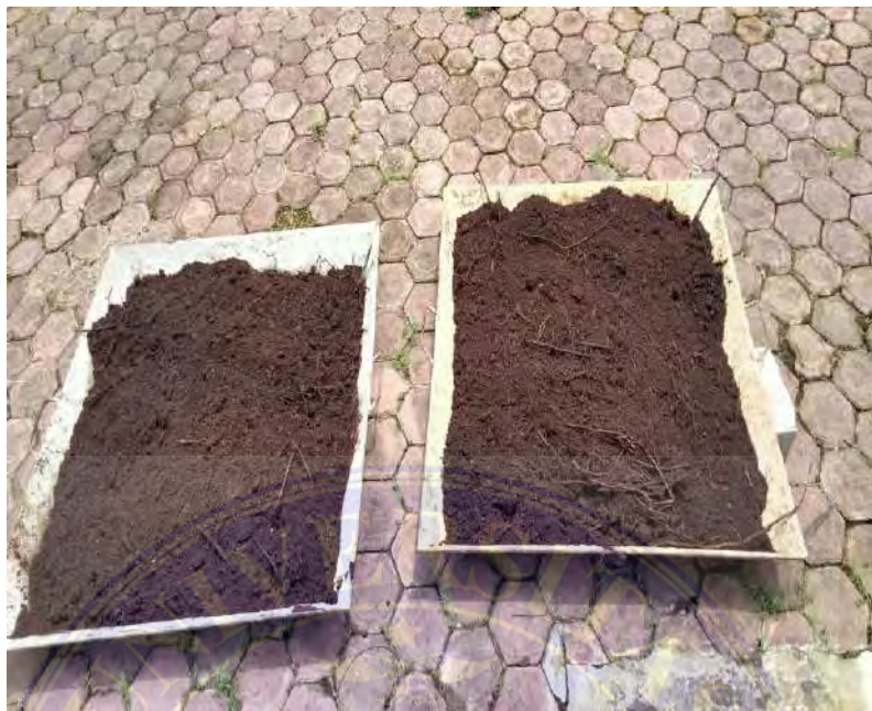
Tanah Gambut Proses Penjemuran Sample
