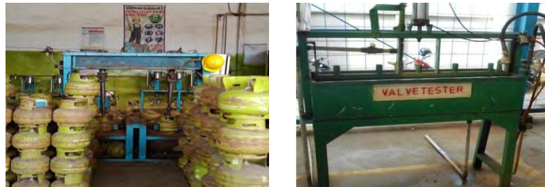
Gambar 2. Fitting Valve Machine Dan Valve Tester
