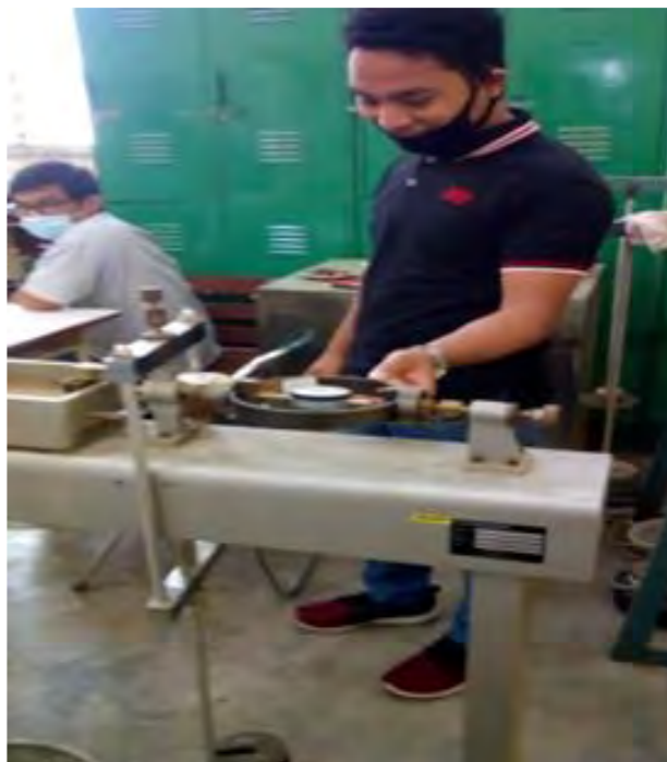
Pengamatan putaran dial direct shear test sample satu
