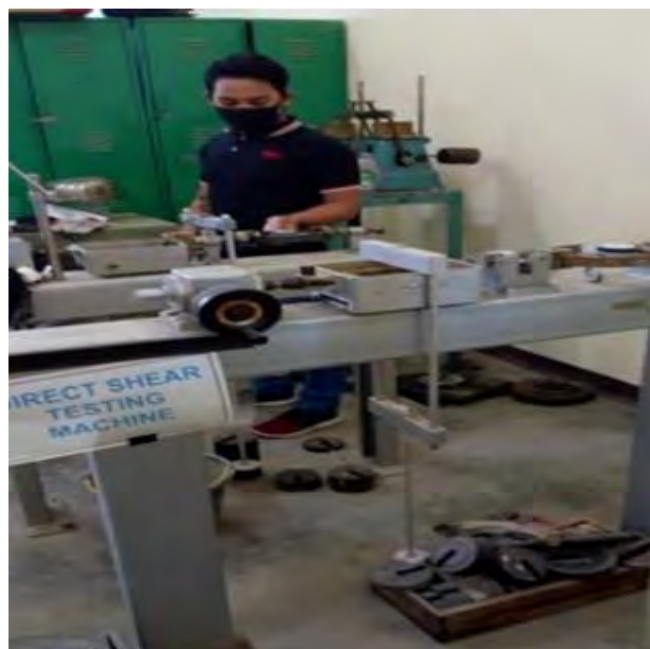
Pengamatan putaran dial direct shear test sample dua
