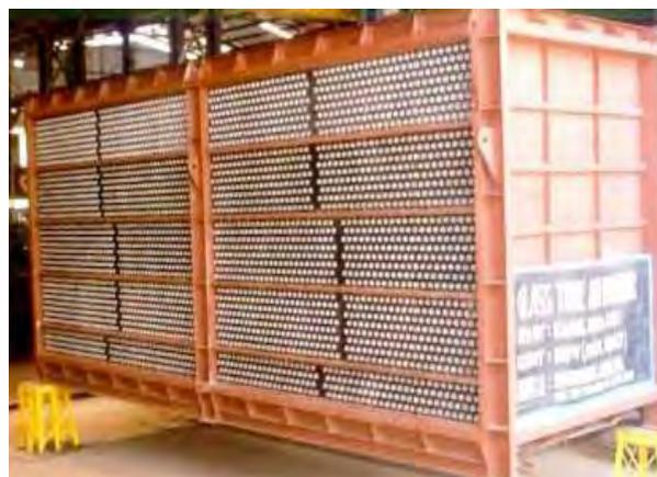
Gambar 2.10. Tubular type *Air priheater*
