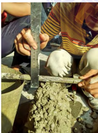
Mengukur Nilai Slump
