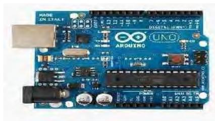
**Gambar 2.4 Modul Arduino UNO**
