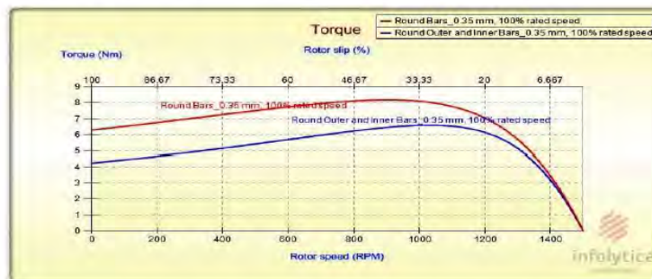
Figure 6: Torque vs. Speed for Two (2) type of Rotor Bar
