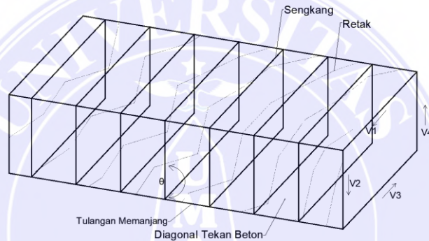
Gambar 3.6.c Space truss analogy
