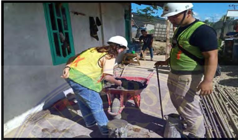
Gambar 4.9 Proses Uji Slump Test
