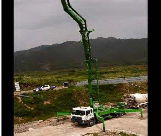
Gambar 3.8 (cp) *concrete pump*
