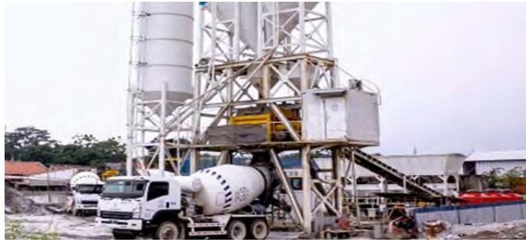
Gambar 4.53 *Batching Plant*
