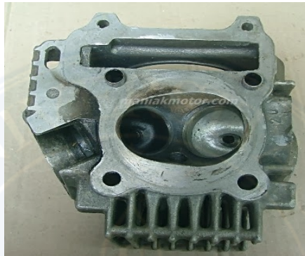
Gambar 2.13 Kepala Silinder (Cylinder Head)
