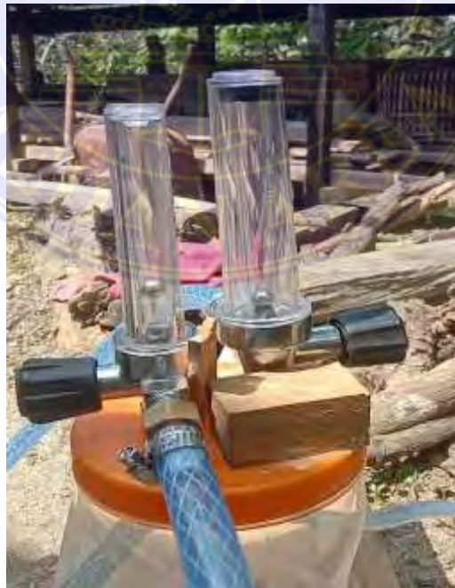
Gambar 3. 2 Flow Meter Gas
