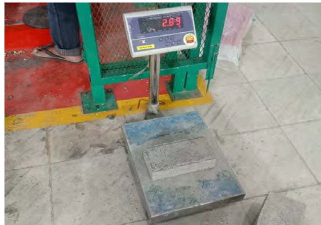
Penimbangan benda uji paving block
