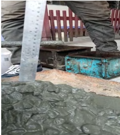
Test Slump Beton
