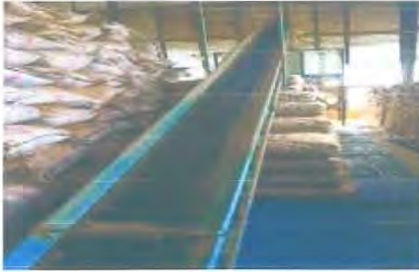
Gambar 3. 36 Conveyor Belt Stair
