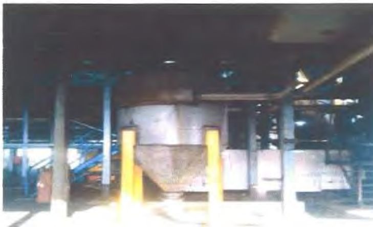
Gambar 3.4 Sand Trap Tank
