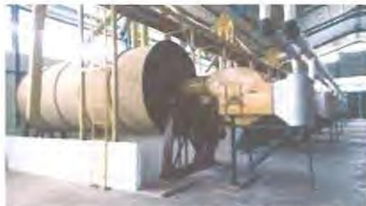
Gambar 3.1. Mesin Drum dryer
