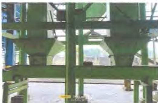
**Gambar 24. Ligh tenera dry separating (LTDS-2)**
