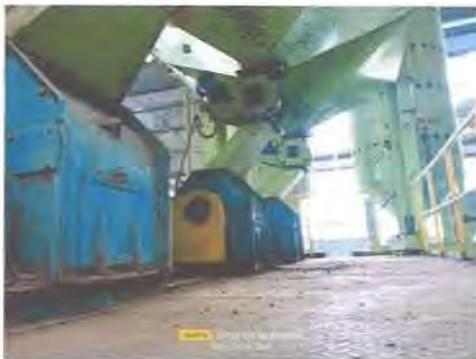
**Gambar 21. *Ripple Mill***
