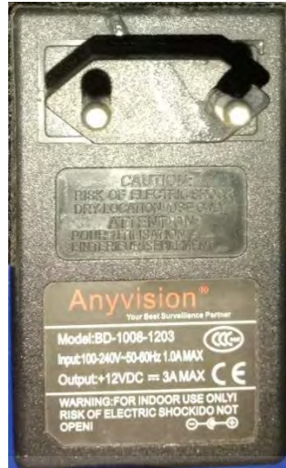
Gambar 3.5 : Power Supply 12 VDC
