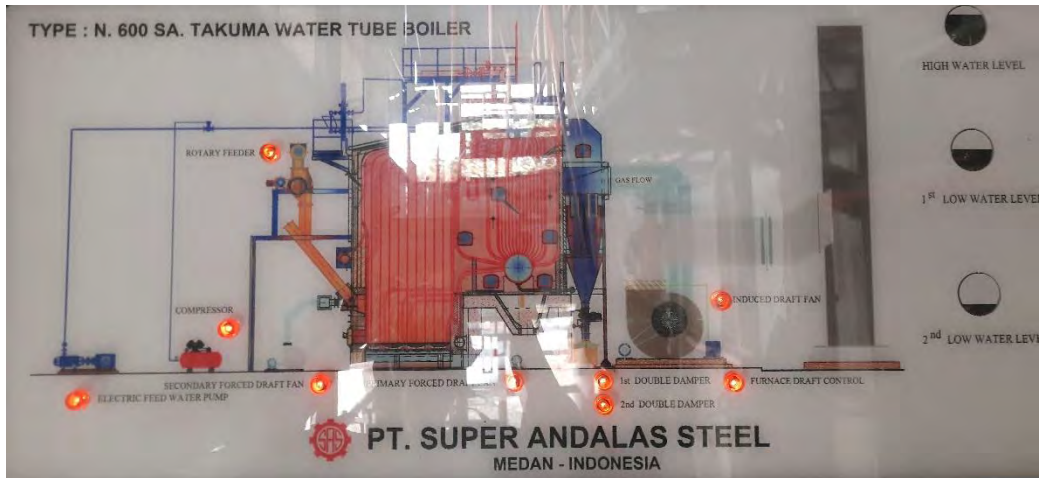
Gambar 3. 1. Boiler PKS Pagar Merbau
