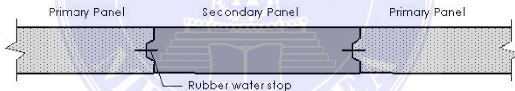
Gambar 2. 9 Dinding diagrama wall Sumber : SNI 8460:2017
