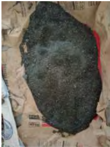
Abu boiler pabrik kelapa sawit
