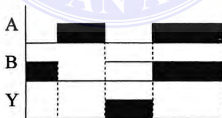
Gambar 3.11 Timing Diagram Gerbang NOR
