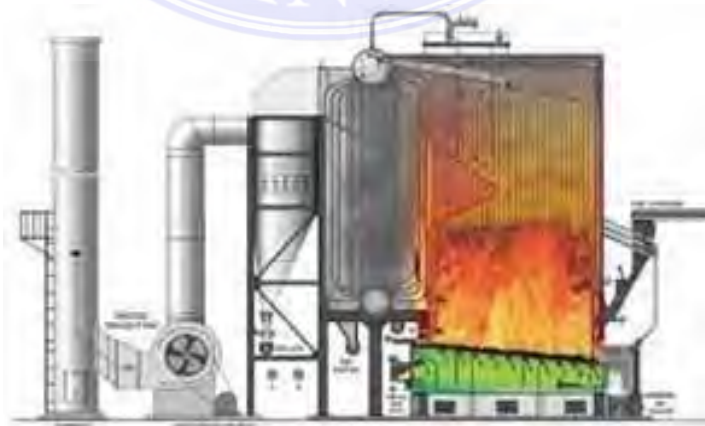
Gambar 2. 5 Circulating Fluidized Bed Boiler
