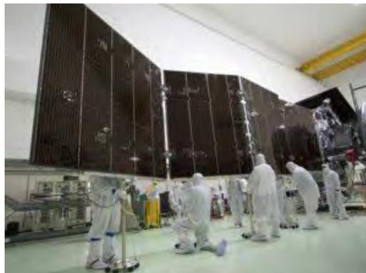
Gambar 2.5 Panel Jenis *Compound Thin Film Triple Junction Photovoltaic*
