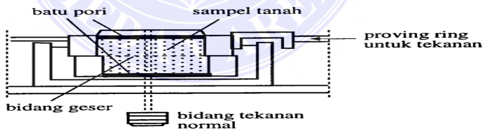
Gambar 5. Adventure is out there: direct shear test (Uji kuat geser batuan),(Hary Chrstady, 2011)
